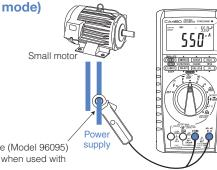
AC/DC clamp-on probe (Model 96095) Reads maximum 60 A when used with the CA450.
